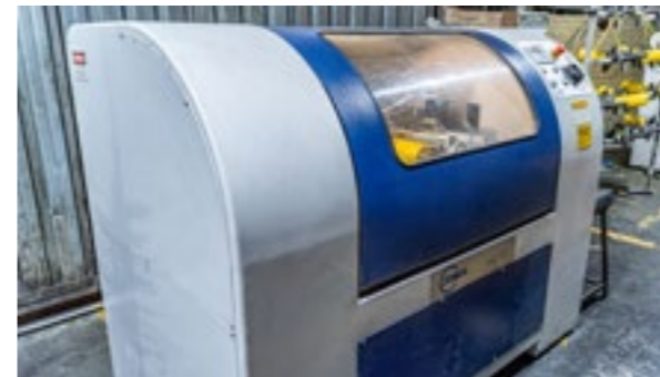
Twister machine that makes baling twine
