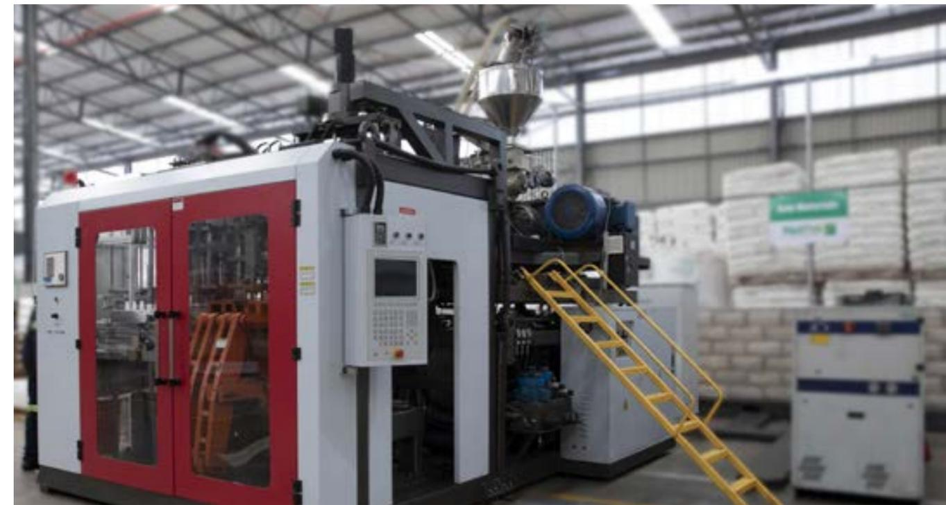
High Density Polyethylene (HDPE) bottle blowing machine
