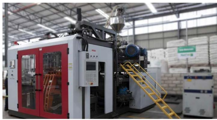
High Density Polyethylene (HDPE) bottle blowing machine
